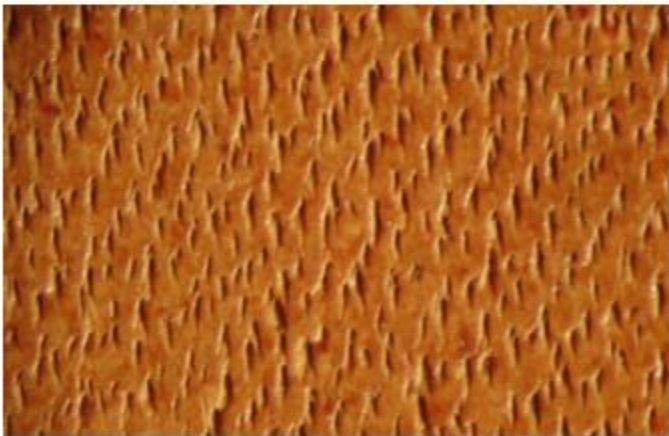
Grain surface of a leather sample
