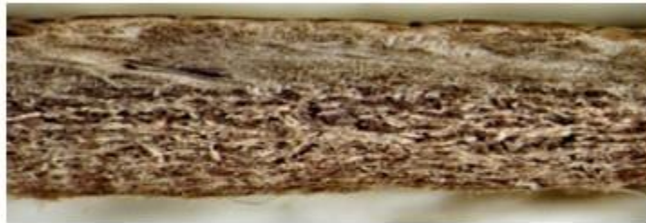
Section of leather from wool-bearing sheep showing delamination.
