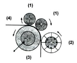
Knife cylinder and transport rollers.
