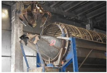
Desalting cage and enclosed conveyor for drum feed.
