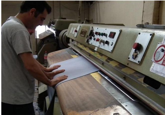
The butt part is presented grain down using a feed roller (*or table*).
