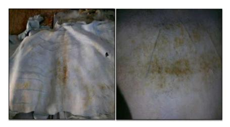
During drying of leathers, fungi may also develop, since favourable conditions with respect to humidity and temperature can arise inside the drying chambers. Bio-deterioration becomes visible as spots of various sizes in green, yellow-brown, dark-brown, grey and brown-green shades. Major microbial damage to tanned and finished leathers and products is caused by fungi as shown below.
